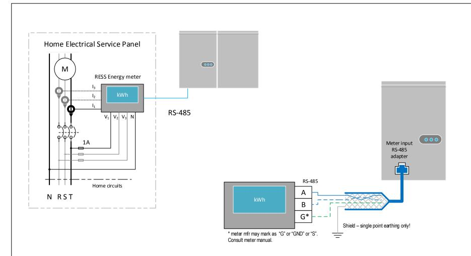
Energy meter supports 1Ø and 3Ø configuration. 3Ø service shown. For 1Ø service, do not populate R,S ph components.
