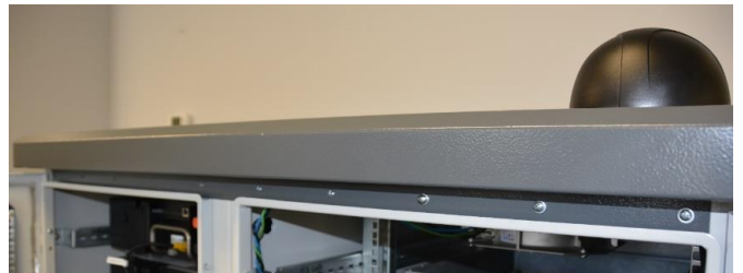
Figure 7: Fastening the canopy to the cabinet.
