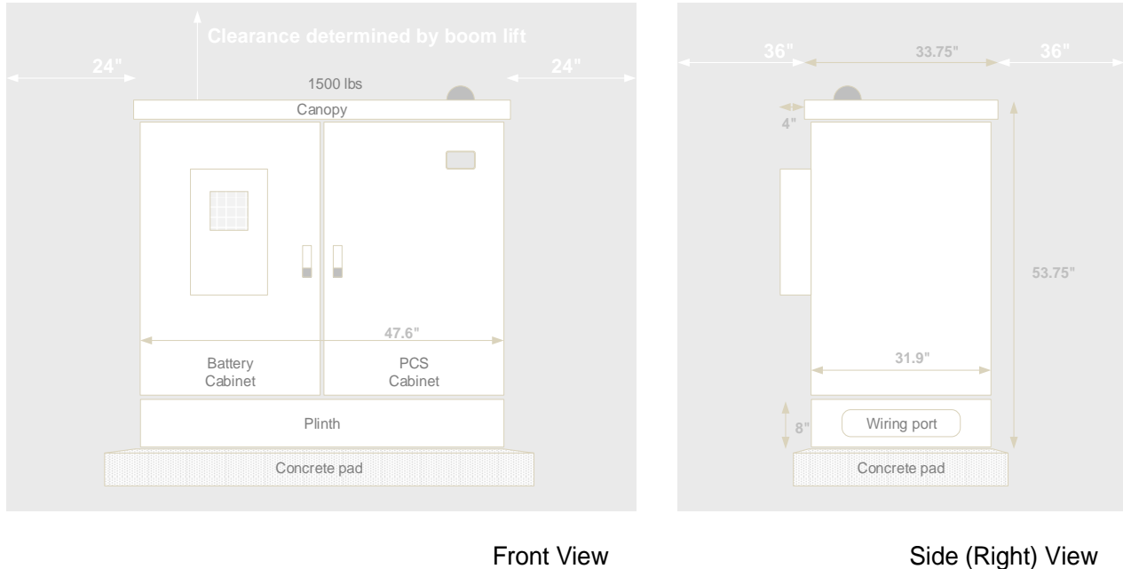
Figure 1: Mounting installation plan – minimum clearances required for installation and service access to the battery system.
