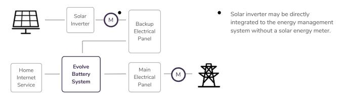
The system may be installed in a manner differently than shown above. In addition, in accordance with the local electrical code, the installer may have included dedicated emergency disconnect switches for the battery and solar inverters. Consult your system installer regarding the application and installation setup of your specific system. Refer to the Installer Checklist at the end of this document regarding information to be provided to you from your certified system installer.
