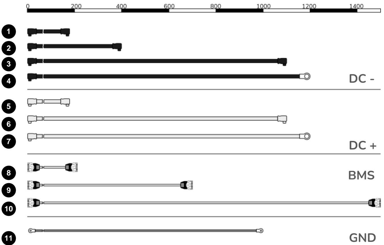
Figure 28: Expansion cabinet cable kit.
